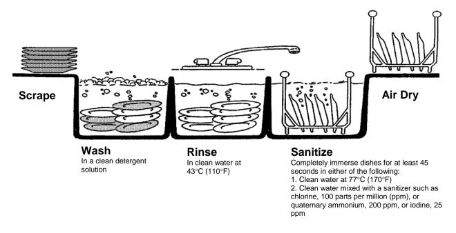
Utensils for preparing food can be washed, rinsed, and sanitized in a 2 compartment sink. The washing and rinsing would occur in the first sink, with sanitizing occurring in the second sink.
