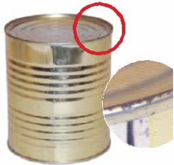
Pitted rust or leaking
