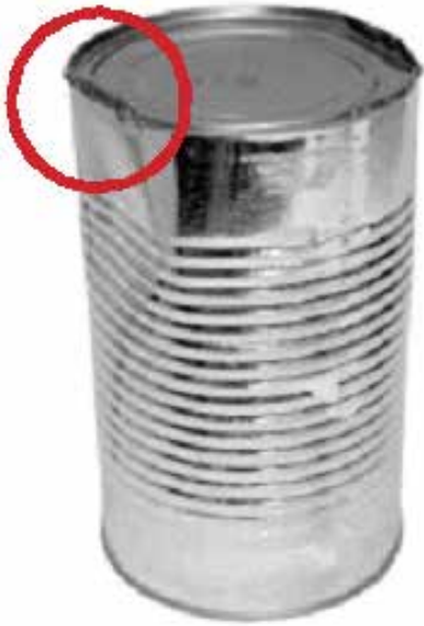
Dented at junction of side and end
