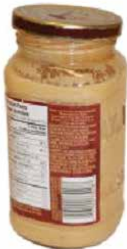
Crooked lid, vacuum button raised, other evidence that cap has been opened
